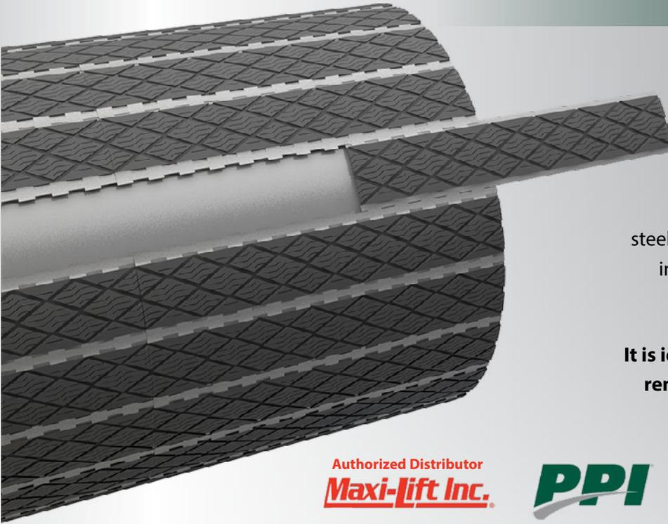
**EZ-LAG™** is a field replaceable lagging that's bonded to a 5" wide steel backer, similar to Craft-Lag. However, unlike Craft Lag, EZ-LAG has perforations in the steel backer that allow it to be formed to in the field fit any pulley diameter 12" and over.
