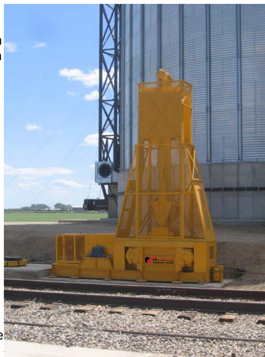
MODEL 100/125 WITH DTC DRIVE 45,000 lbs LINE PULL
